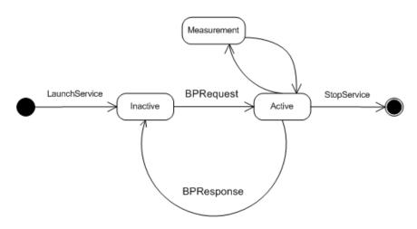
Figure 5.3: Blood pressure service state machine
