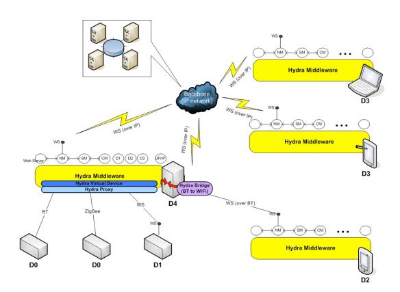
Figure 2.1: Device integration in Hydra
