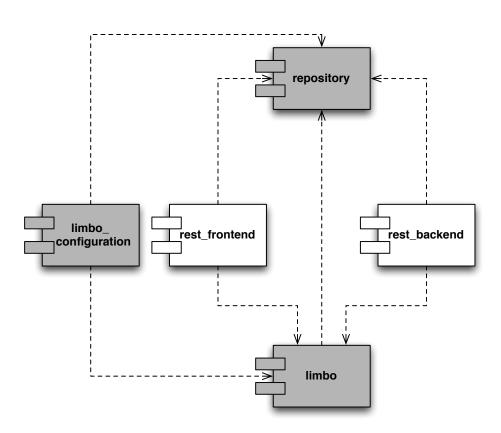
Figure 3.3: Component diagram of REST deployment
