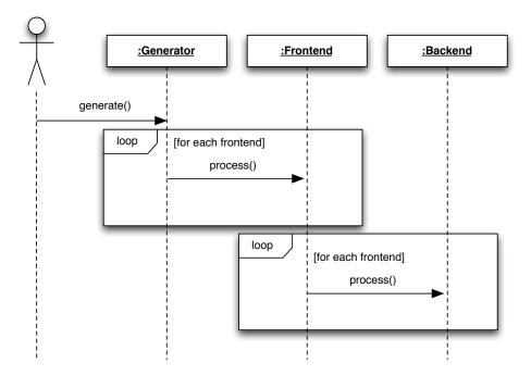
Figure 3.4: Sequence diagram of Limbo control flow
