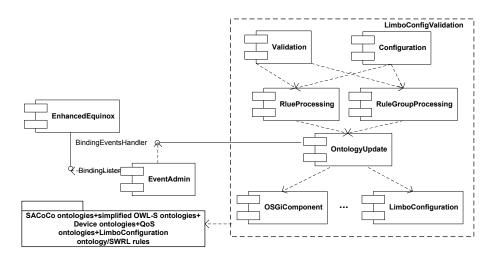
Figure 8.2: Limbo configuration and validation prototype architecture
