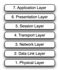
Figure 2.1: The seven layers of the OSI reference model.
