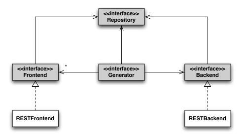
Figure 3.2: Class diagram of Limbo REST implementation
