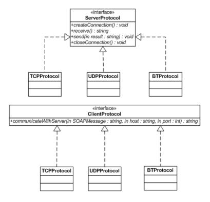
Figure 2.12: Class diagram for Protocol support in Limbo.
