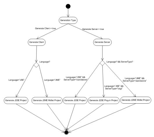
Figure 4.1: Activity diagram for project generation feature
