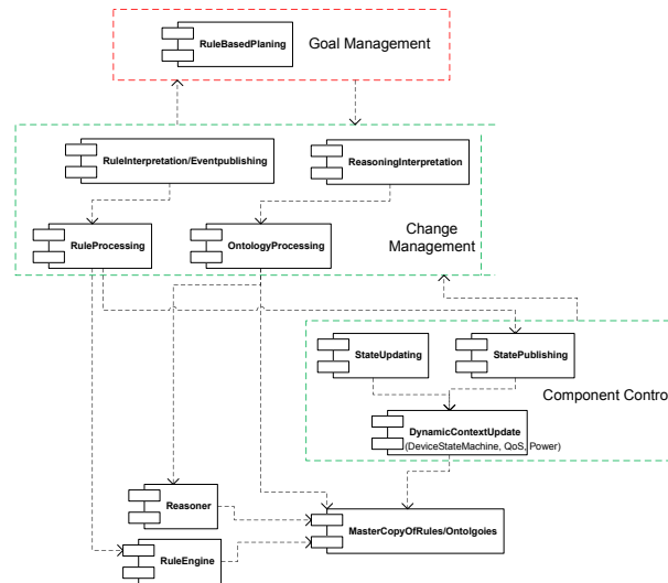
Fig. 1. Architecture of the self-management in Hydra
